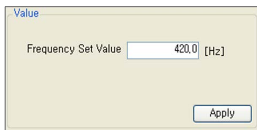
图 12.3-6 运行频率设置 (Motor Drive:High Speed Induction Motor)
